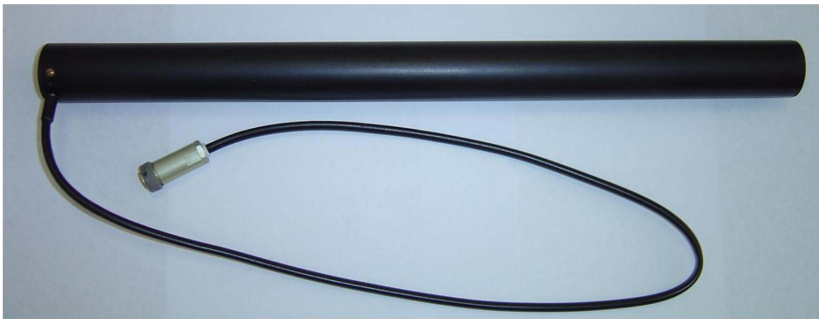
Figure 2. EGLE magnetometric probe MH with 0.7m cable connected.
